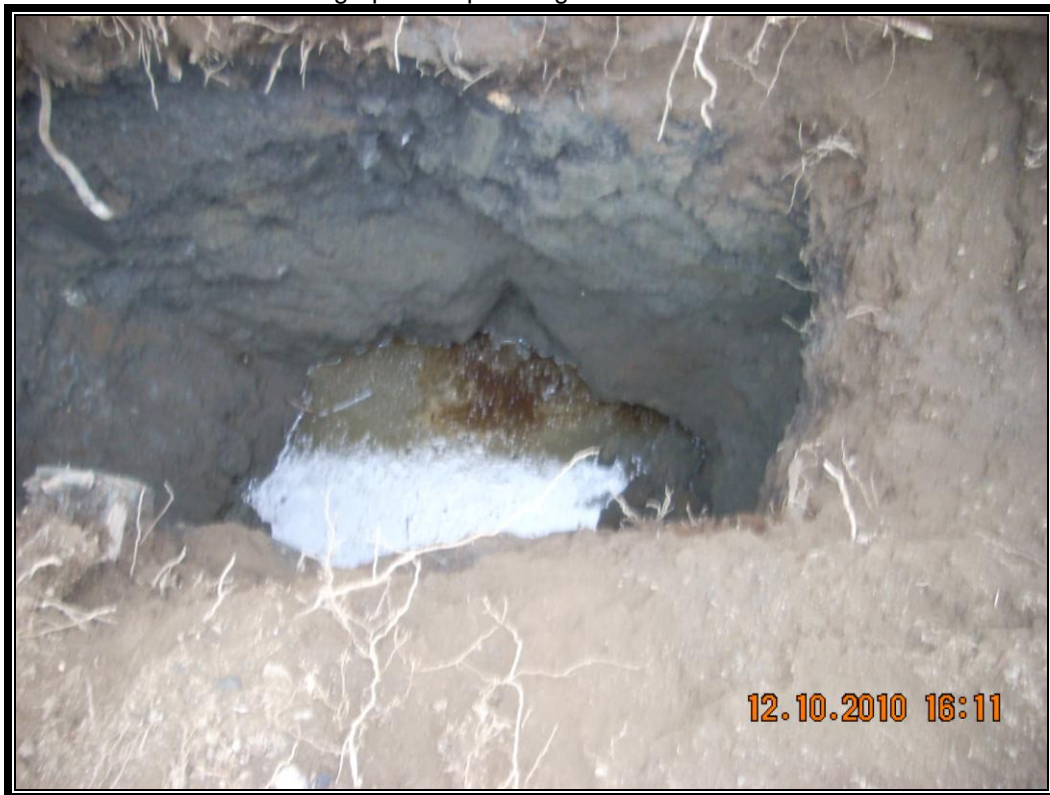
Photograph of free phase fuel oil and impacted soils at TP-8
