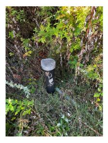
Photo 2 Typical Site groundwater monitoring wells.
