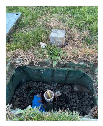
Photo 2: Groundwater Monitoring Well MW-20
