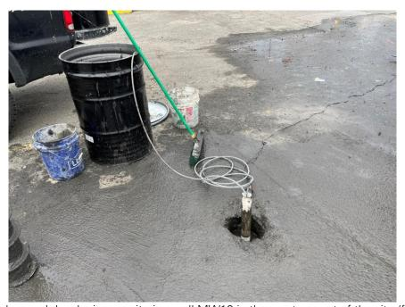
Photo 2: Lakewood developing monitoring well MW19 in the western part of the site (facing east)
