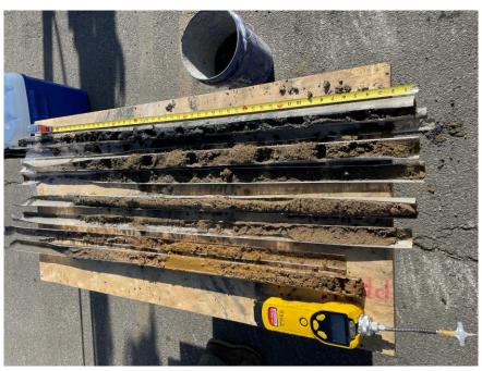
Photo 1: View of soil/fill recovered from soil boring SB24 in the north-central part of the site.
