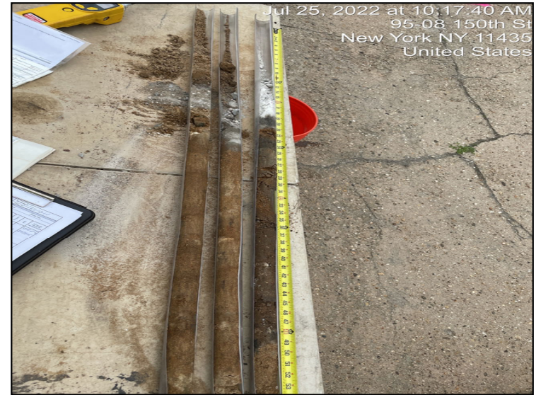
Photograph 2: Soil cores obtained from the Geoprobe at boring location RI-SB-10.
