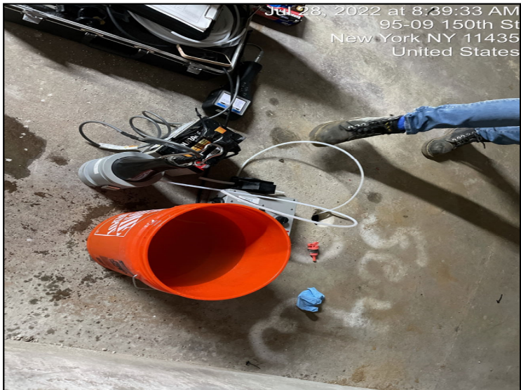
Photograph 7: Purging groundwater from RI-MW-04 during well development activities.
