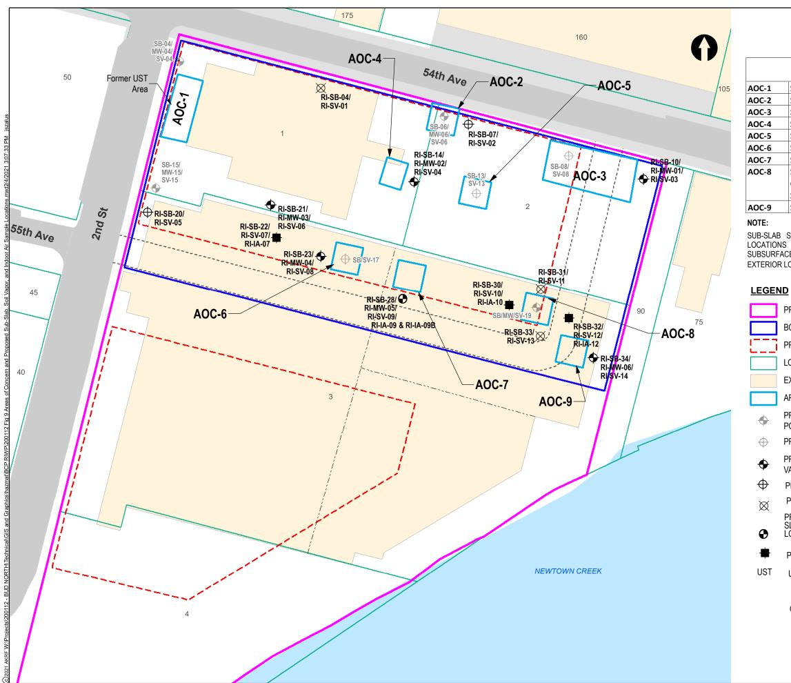
Soil - Elevated Metals. Possible UST Soil - Elevated PAHs, Metals (potentially hazardous) Soil - Elevated PAHs, Metals (potentially hazardous) Soil - Elevated PAHs Soil - Elevated Metals Soil - Elevated Metals (potentially hazardous) Soil - Elevated Metals (potentially hazardous) Soil - Elevated PCBs, PAHs Groundwater - Elevated Freon Soil Vapor - Low level PCE and Elevated Freon
