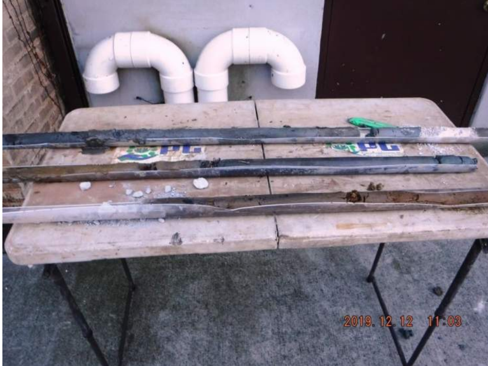
Photograph 5: Soil samples collected from B1. Discoloration by petroleum is evident (grey-colored material).
