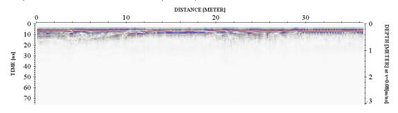
**Step 3.** Correct for attenuation losses (energy decay function)
