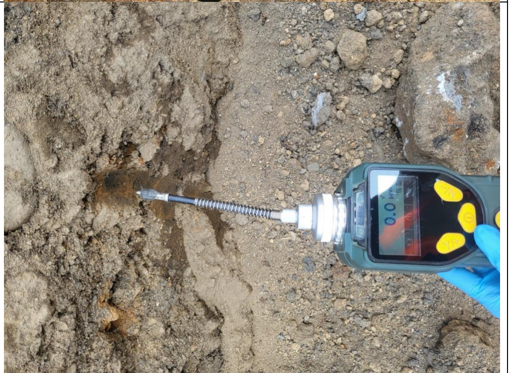
Photo 4 – PID reading at the soil next to the UST.
