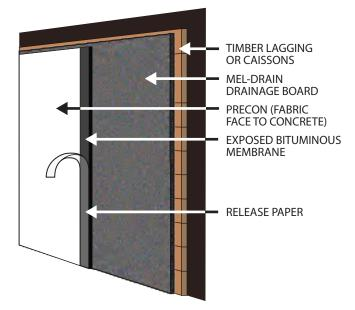
2. Overlap the edge of the subsequent sheet. Roll press into place to ensure good adhesion.
