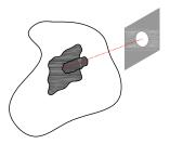
Cut a piece of DETAIL FABRIC 4. to the dimensions of the soil nail plate and embed the fabric into the previously applied HYDRALASTIC 836.
