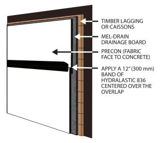
4. Ensure that DETAIL FABRIC is centered over the termination with 6" (150 mm) on each side of lap edge. Press DETAIL FABRIC into place to ensure that the HYDRALASTIC 836 has fully wetted out the fabric.
