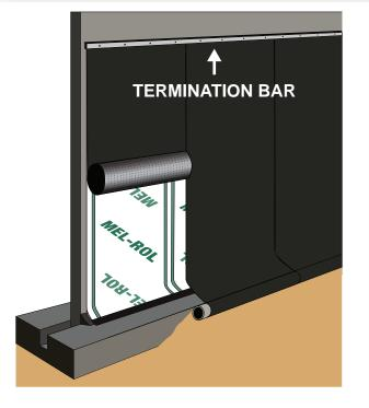
Backfilling should be done immediately, using care and caution to avoid damaging the water-proofing application.
