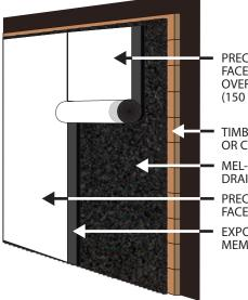
PRECON (FABRIC FACE TO CONCRETE) OVERLAPPED 6" (150 mm)
