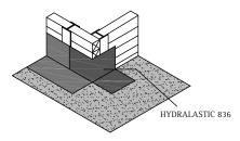
**3.** Apply HYDRALASTIC 836 to all overlap areas of PRECON that will be accepting the subsequent sheet of PRECON.
