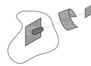
5. Cut another two pieces of DETAIL FABRIC, one for the shaft of the soil nail, the other for the top, and embed this fabric into the previously applied HYDRALASTIC 836.
