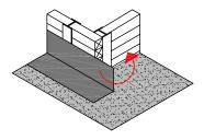
Install PRECON according to installation instructions onto soil stabilization system. Allow a minimum of 12" overlap to extend around outside corner.
