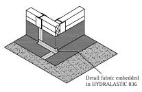
**6.** Apply HYDRALASTIC 836 at all overlapping joints in a 12" wide application and then fully embed detail fabric into this HYDRALASTIC 836. Terminate all edges with additional HYDRALASTIC 836.
