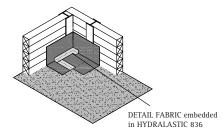
**5.** Apply HYDRALASTIC 836 at all overlapping joints in a 12" wide application and then fully embed DETAIL FABRIC into this HYDRALASTIC 836. Terminate all edges with additional HYDRALASTIC 836.
