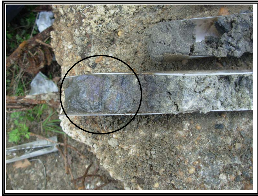
Photo 5: View of soil core from soil boring SB-22, showing petroleum sheen (circled) within saturated gray sand (8.5 feet below grade).
