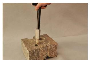
Figure 8. Extracted Vapor Pin<sup>TM</sup>.
