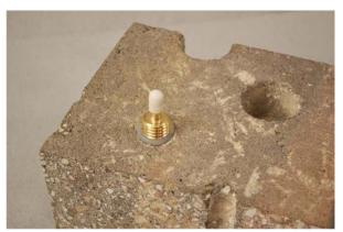
Figure 4. Installed Vapor Pin<sup>TM</sup>.
