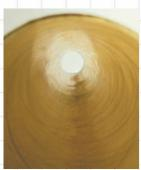
Smooth ID helps reduce the rate of solid buildup inside the casing.
