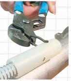
Removing the spring clip allows for easy disassembly of the float.
