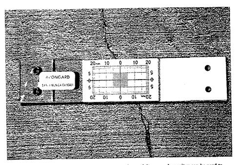
Figure 2. With advanced notice of adjacent construction activity, a crack monitor can be used to determine whether existing cracks in the historic building are stable or still experiencing movement. Compared with measurements taken during the monitoring phase, such information can help determine if subsequent movement resulted from work on the neighboring site. Photo: Avongard Products U.S.A., Ltd.
