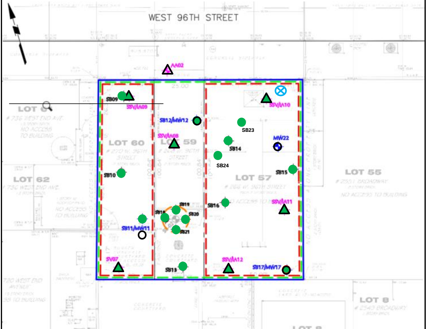
FIGURE 1: BORING LOCATION PLAN
