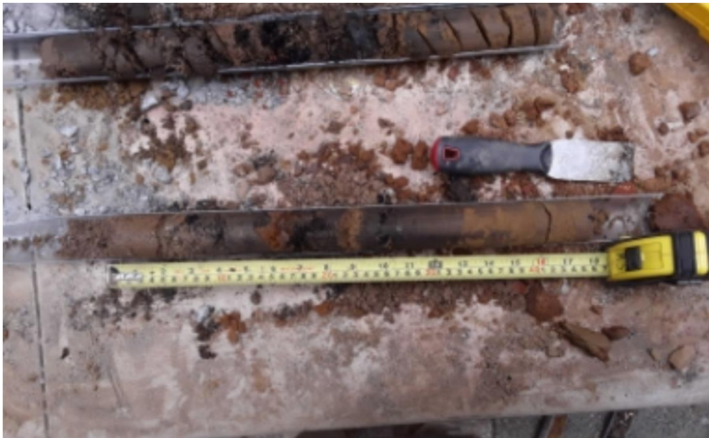
Photo 2: View of odorous and stained material in SP18 from 7 to 8 feet bsg (facing east).
