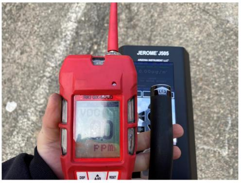
Photo 13: View of the RKI GX-6000 PID and Jerome® J505 used for work zone and ambient air screening (02/12/2022)
