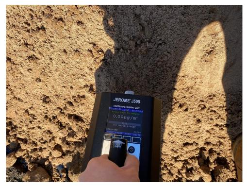
Photo 4: View of Langan screening excavated soil/fill from test pit TP01 using a Jerome<sup>®</sup> J505 mercury analyzer (02/12/2022)
