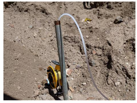
Photo 33: View of tubing in well point used to collect groundwater sample, facing northwest (6/24/2019)
