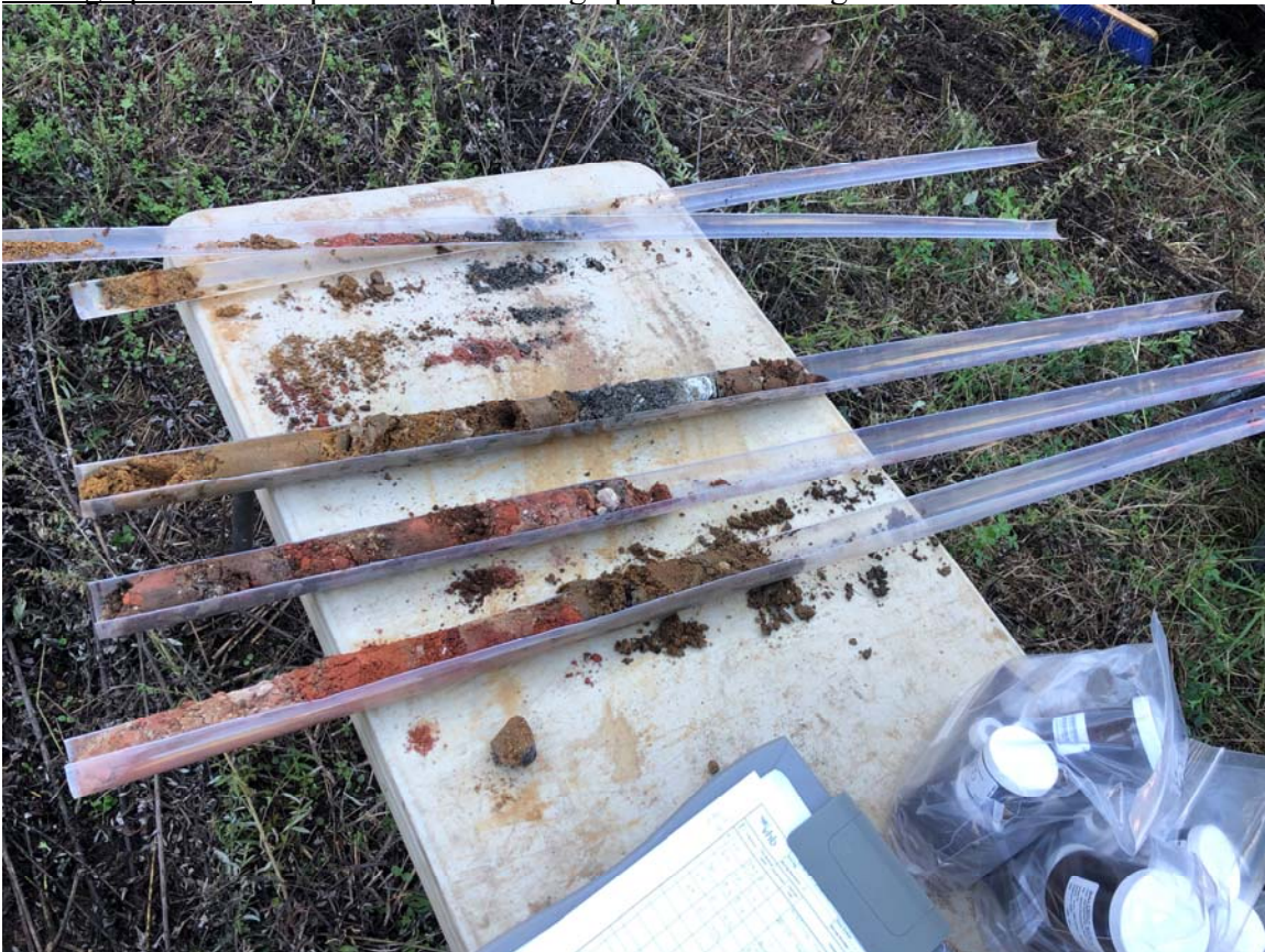
Photograph No. 2: Representative photograph of macrocore samples, with fill material horizons observed in mid-range samples throughout the Site.
