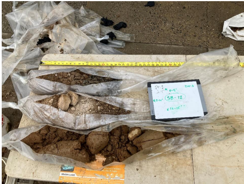
Photo 2: View of soil boring from SB-12.
