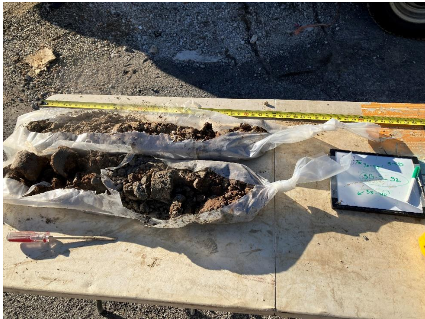
Photo 2: View of soil boring from SB-3_S2 (depth: 30-40 ft bgs).
