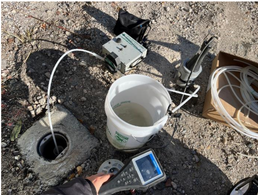
Photo 2: Langan purging groundwater monitoring well MW10 (facing down).
