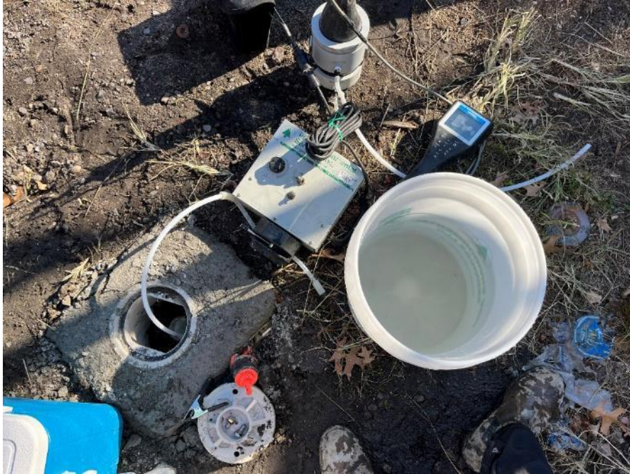
Photo 1: Langan purging groundwater monitoring well MW23 (facing down).
