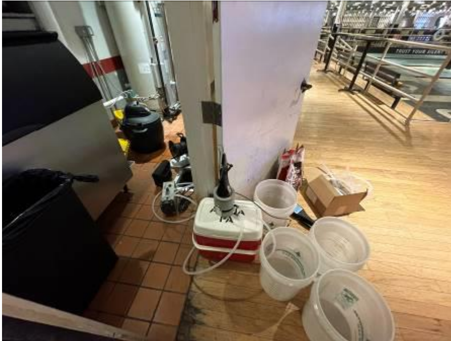
Photo 1: Groundwater sampling setup at monitoring well MW08D (facing west).
