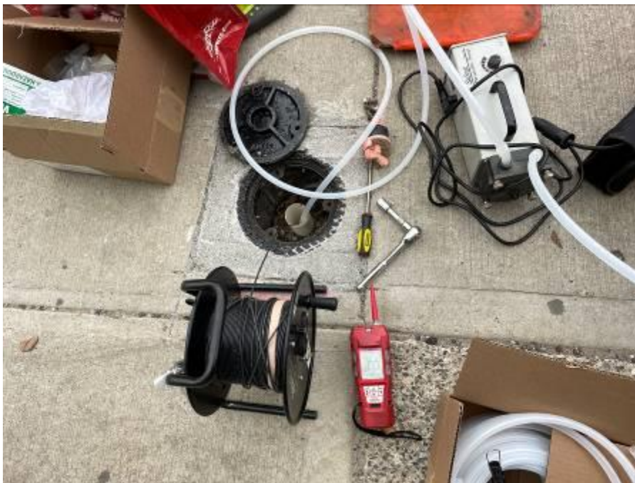
Photo 2: Groundwater sampling setup at monitoring well HRP-MW-1.
