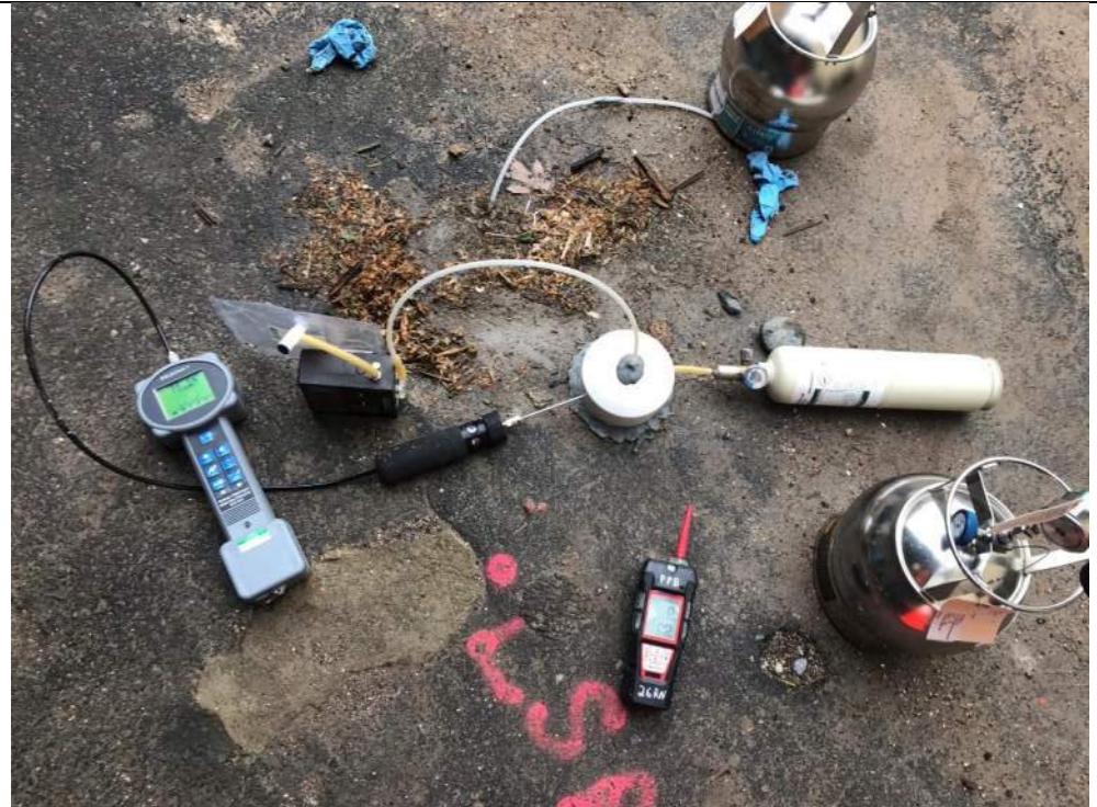
Photo 2 – Helium leak detector test prior to soil vapor sampling, facing south.
