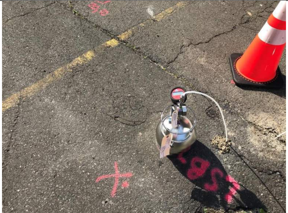
Photo 3 – Soil vapor sampling collection at LSV-5A into 6 Liter Summa canisters, facing north.
