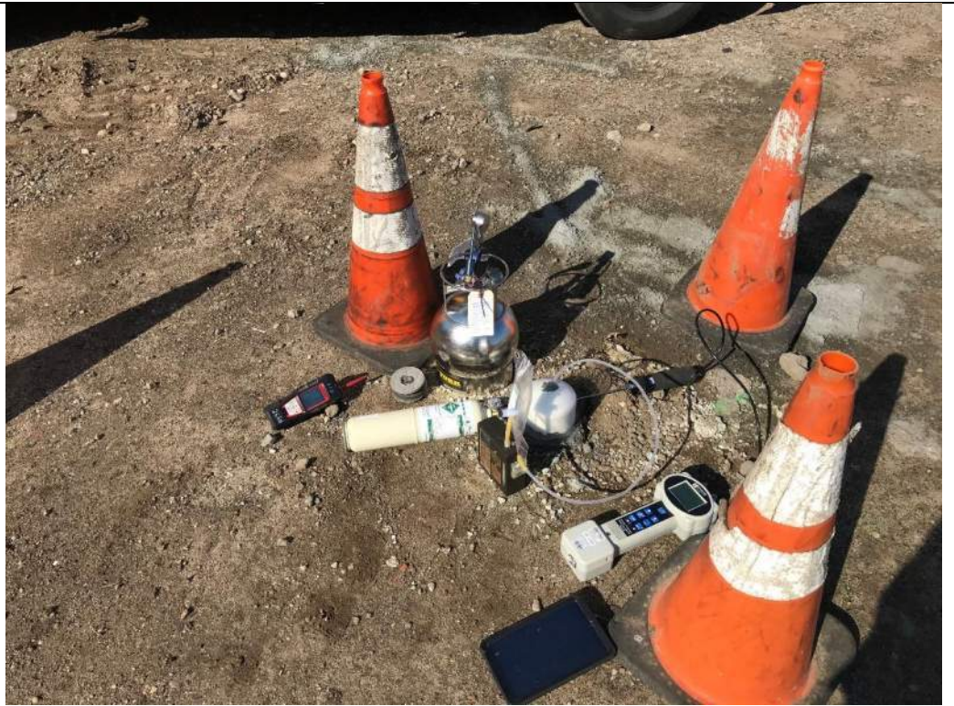
Photo 2 – View of helium leak testing prior to soil vapor sampling at LSV-2, facing southwest.
