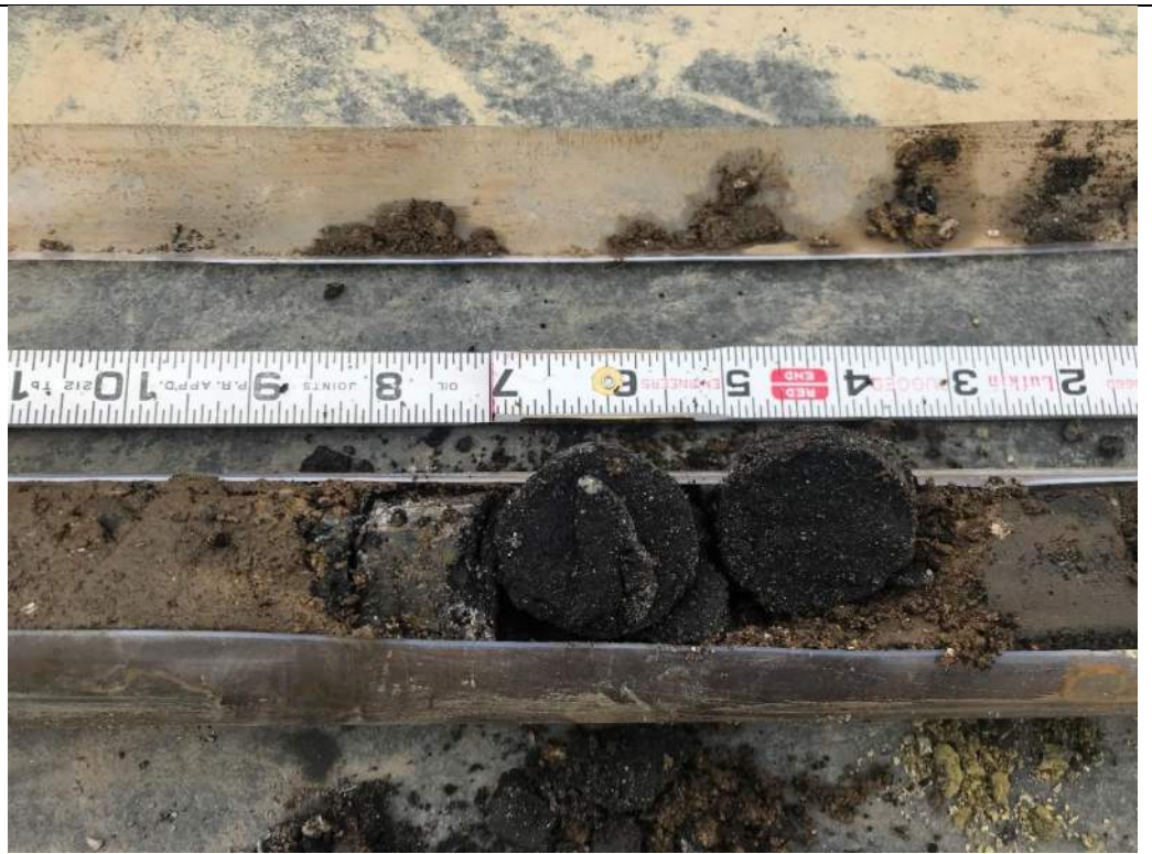
Photo 2 – Ash layer identified in LSB-24 from 4 to 4.5-feet bgs.
