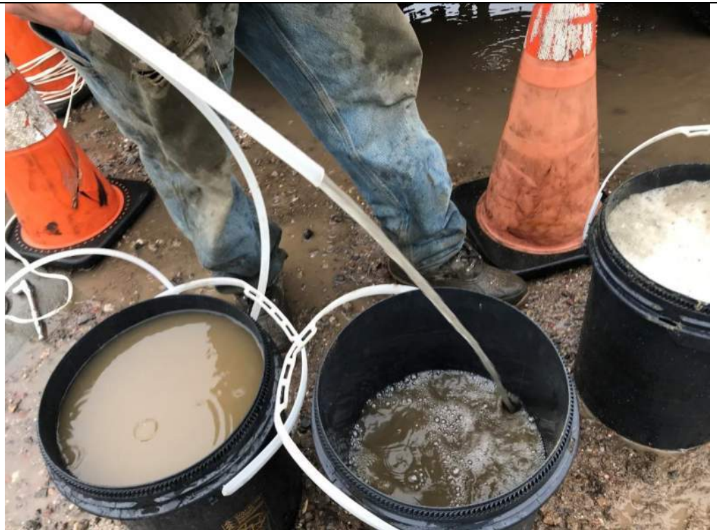
Photo 4 – Developing monitoring well LMW-14 until discharge ran free and clear of solids, facing north.
