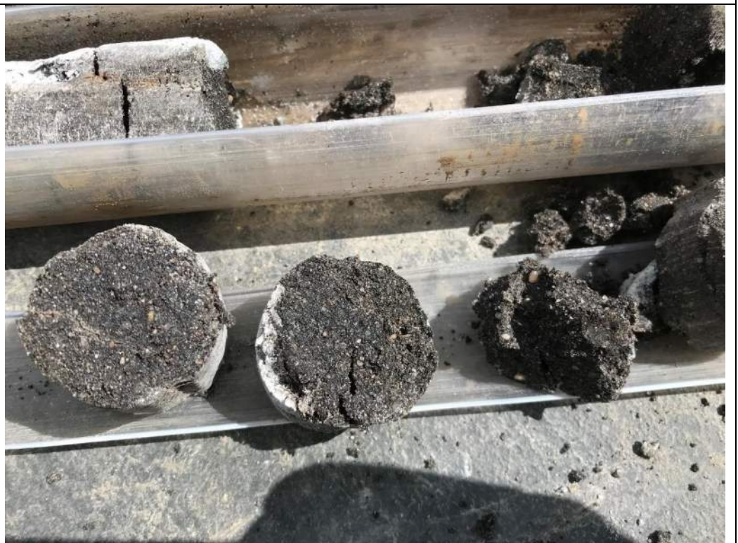
Photo 4 – Ash layer identified in LSB-23 from 8.5 to 10-foot bgs.
