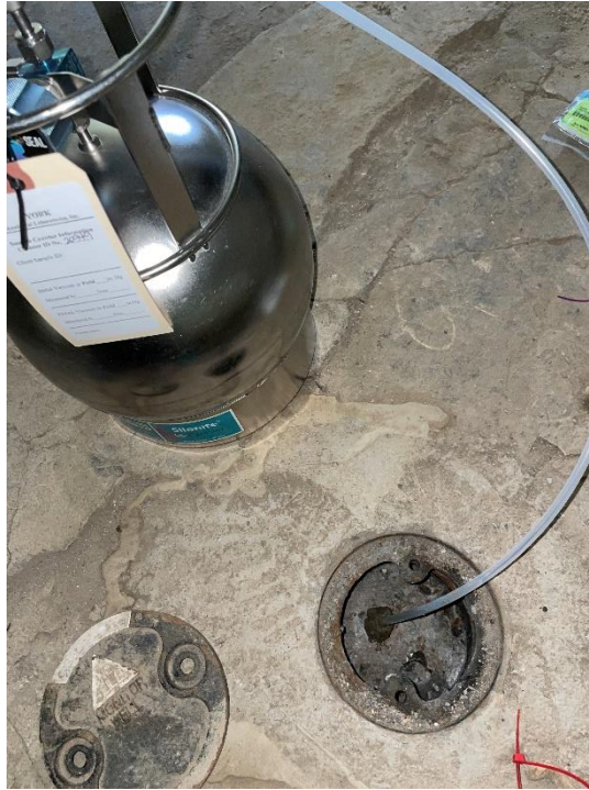
Photo 11, 11/29/2023: Langan collecting soil vapor sample MP01_112923 (facing down).
