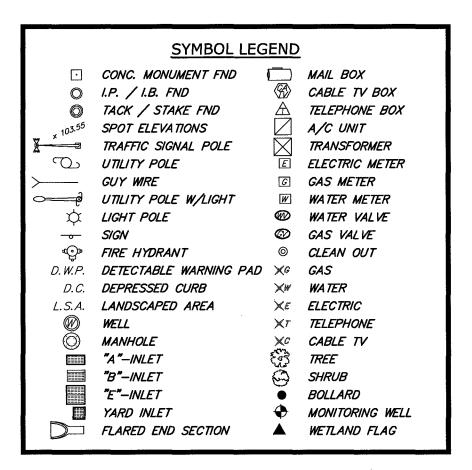
SYMBOL LEGEND CONC. MONUMENT FND © CLEAN OUT **X**<sup>©</sup> GAS CABLE TV BOX TACK / STAKE FND D.C. **DEPRESSED CURB** ×₩ WATER TELEPHONE BOX XE ELECTRIC L.S.A. LANDSCAPED AREA D.W.P. DETECTABLE WARNING PAD A/C UNIT XT TELEPHONE TRANSFORMER XC CABLE TV ELECTRIC METER UTILITY POLE "A"-INLET TREE G GAS METER SHRUB "B"-INLET "E"-INLET WATER METER **BOLLARD** WATER VALVE OFFICE WALIGHT YARD INLET MONITORING WELL FLARED END SECTION O GAS VALVE WELL
