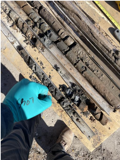
Photo 1: View of recovered soil from WC07.
