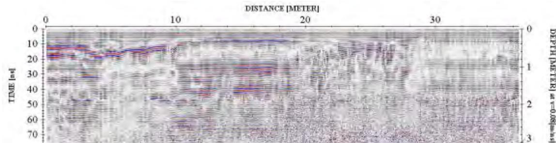
**Step 4.** Remove static from bottom of profile (*time cut*)
