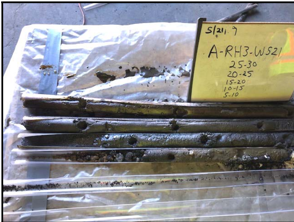
A-RH3-WS21: Close View 1 with Staining at 17 to 23 Feet and 25 to 28 Feet
