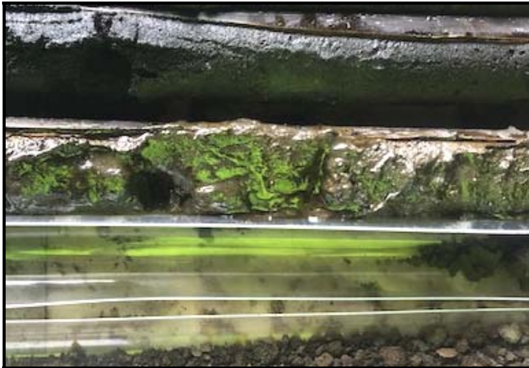
A-RH3-WS25: Close-up of NAPL at 15 to 17.5 Feet (Middle Sleeve)
