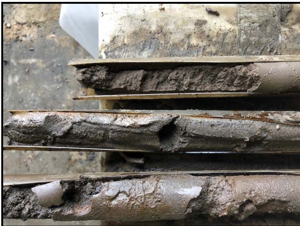
A-RH3-B41: Staining at 20 to 21 Feet
