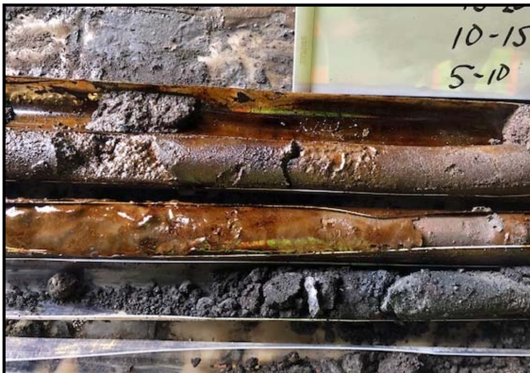
A-RH3-WS17: Close-up of NAPL at 20 to 23 Feet and Staining at 25 to 27 Feet
