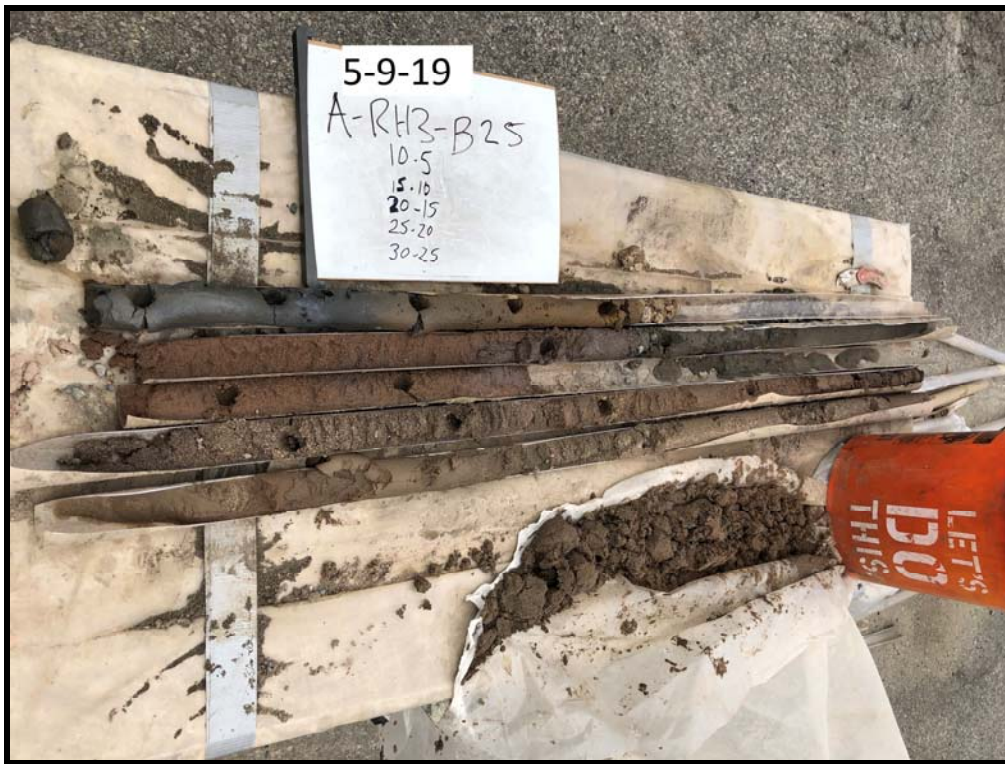
A-RH3-B25: Staining at 7 to 12 Feet
