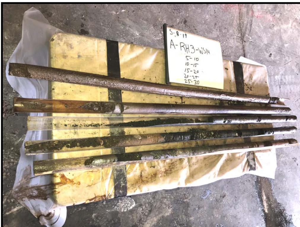
A-RH3-WS14: 5- to 30-Foot Soil Cores with Staining from 15 to 30 Feet
