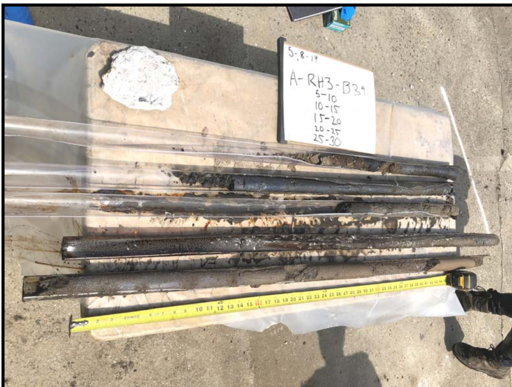
A-RH3-B39: 5- to 30-Foot Soil Cores with Iridescence and Staining at 7 to 15 Feet
