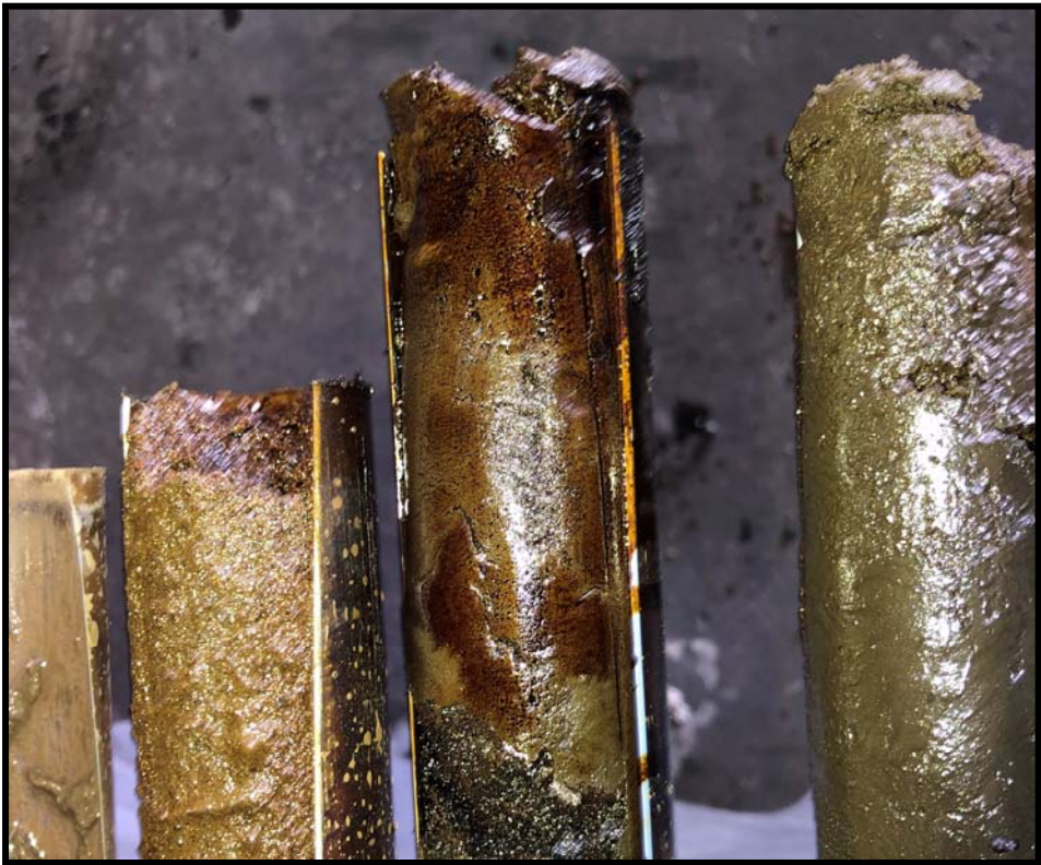
A-RH3-WS14: Close-up of NAPL at 19 to 20 Feet
