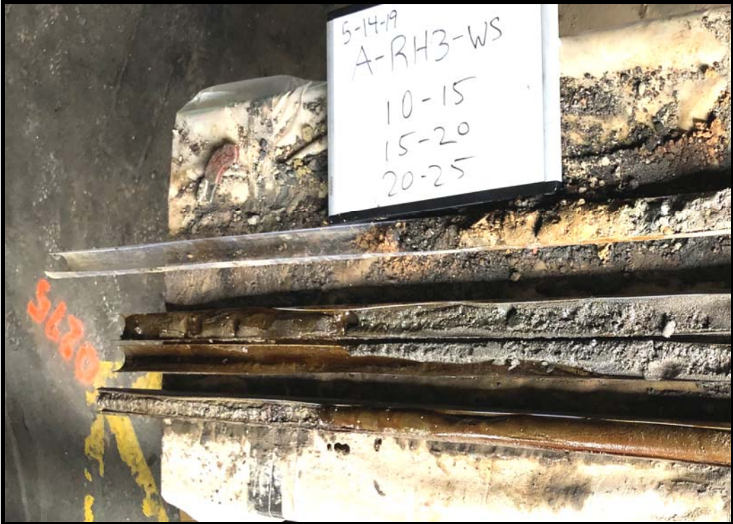
A-RH3-WS20: Close-up of NAPL at 15 to 16 Feet and 22 to 27 Feet
