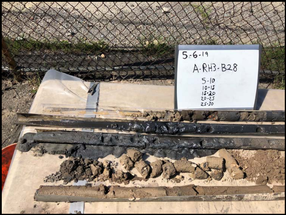
A-RH3-B28: Staining and Slight Sheen at 10 to 14 Feet and 15 to 17 Feet
