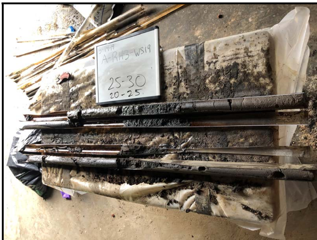
A-RH3-WS19: 20- to 30-Foot Soil Cores Showing Staining at 20 to 29 Feet
