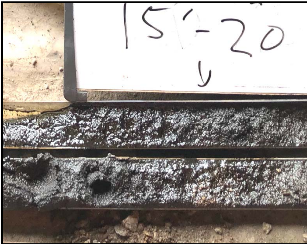
A-RH3-B37: Close-up of Sheen and Staining at 15 to 17.5 Feet
