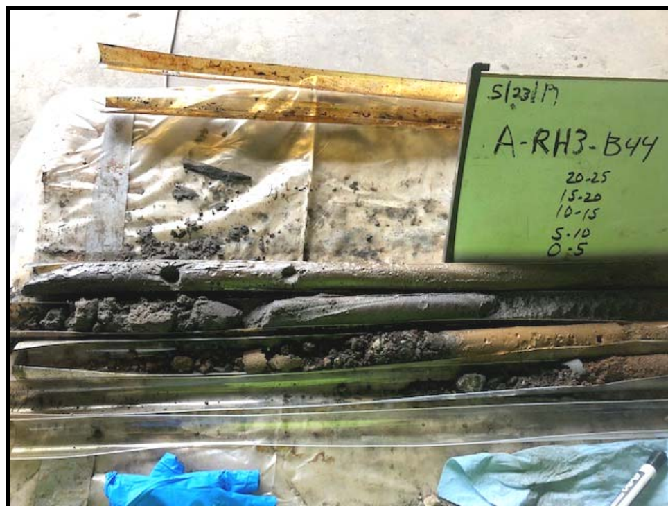
A-RH3-B44: Showing Close-up of Staining in a Portion of 13.5- to 25-Foot Interval
