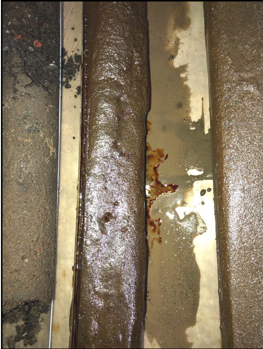
A-RH3-B32: Close-up of Staining and Small Amount of NAPL in 15- to 20-Foot Interval
