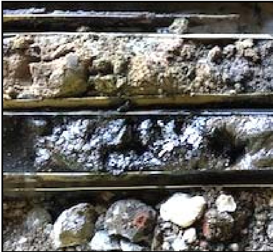
A-RH3-WS24: NAPL at 10 to 11 Feet (Middle Sleeve)
