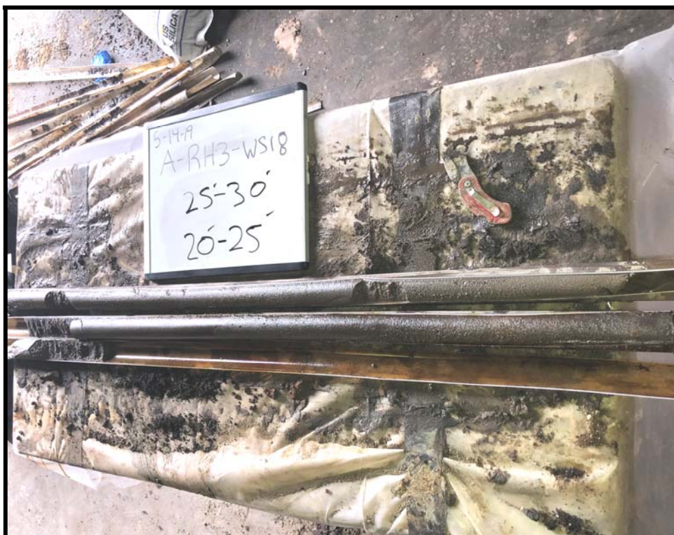
A-RH3-WS18: 20- to 30-Foot Soil Cores Showing Stained Soil and Liner at 20 to 25 Feet
