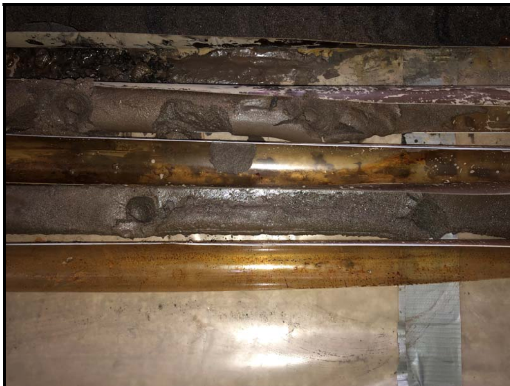
A-RH3-B36: Close-up of Staining from 20 to 30 Feet
