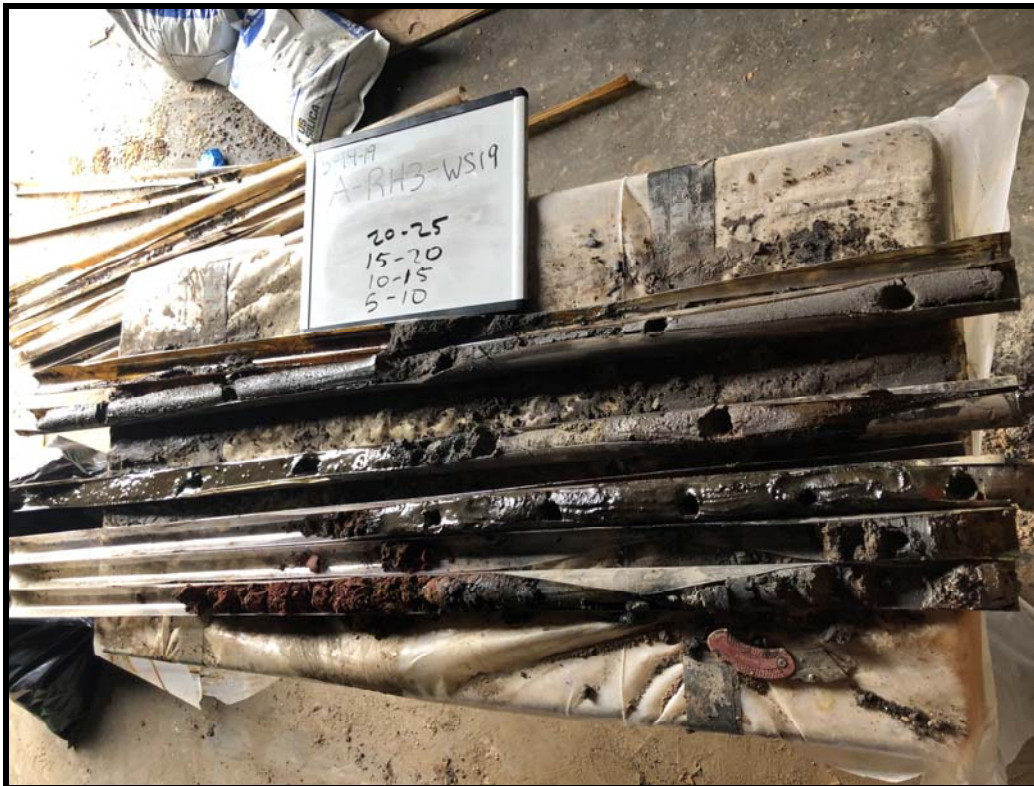
A-RH3-WS19: 5- to 25-Foot Soil Cores Showing Staining 11 to 17 Feet
