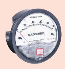
Select the Dwyer® Magnehelic® gage for high accuracy — guaranteed within 2% of full-scale — and for the wide choice of 81 models available to suit your needs precisely. Using Dwyer's simple, frictionless Magnehelic® gage movement, it quickly indicates low air or noncorrosive gas pressures — either positive, negative (vacuum) or differential. The design resists shock, vibration and over-pressures. No manometer fluid to evaporate, freeze or cause toxic or leveling problems. It's inexpensive, too.
