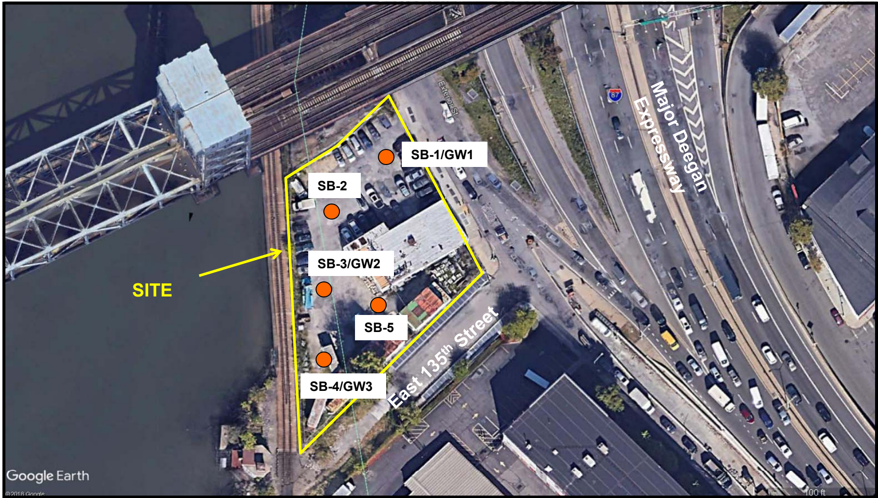
FIGURE 2 - SOIL BORING AND GROUNDWATER SAMPLE LOCATION MAP
