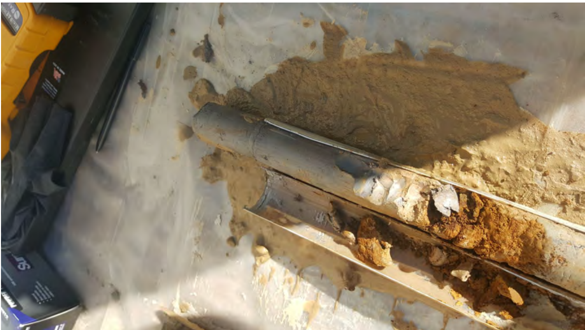
Photo B4 – Core of Clay Layer from SB-12
