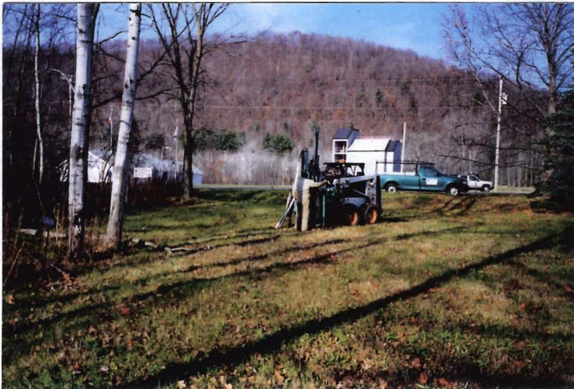
PES Hydrogeologist John Johnson advancing a macro-core soil sample at the location of monitoring well MW-18.
