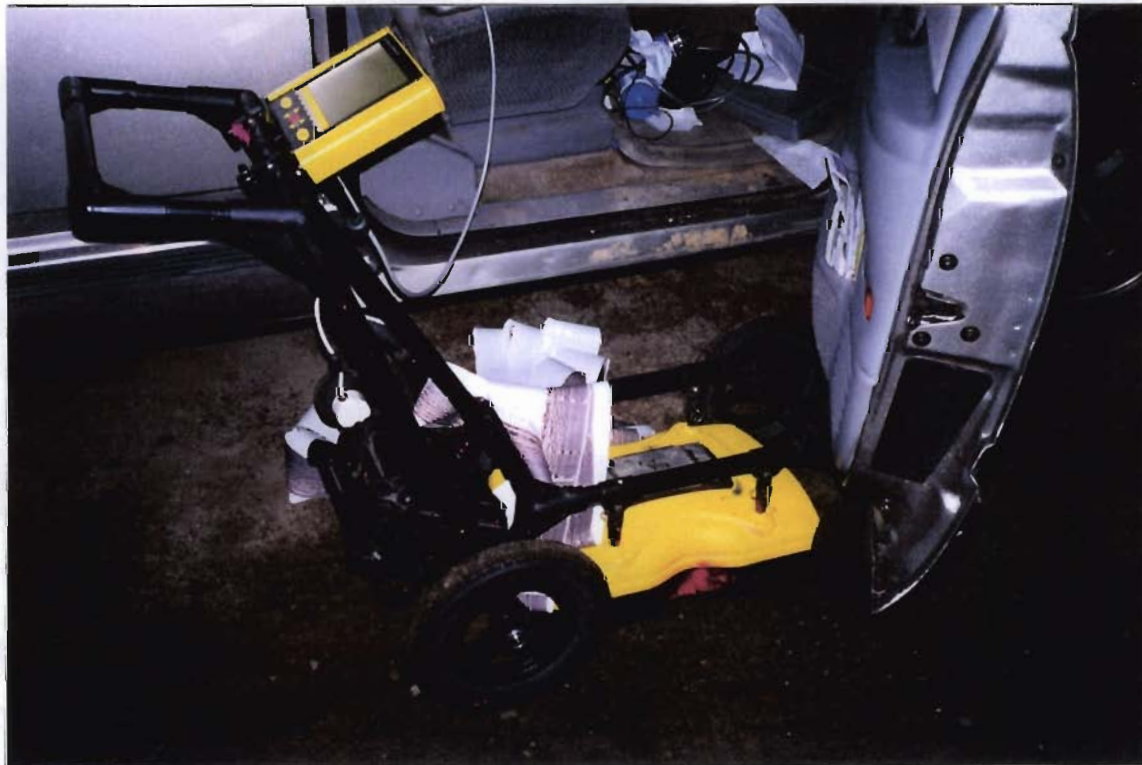
Hager-Richter's Smart Cart Noggin Plus digital subsurface imaging radar system (ground penetrating radar) downloading data to a laptop computer.
