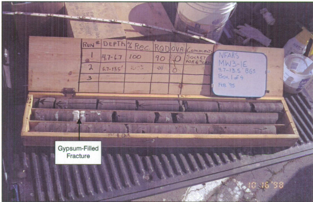
Photo 7 NFARS Rock Core MW3-1E Example of gypsum-filled fracture.
