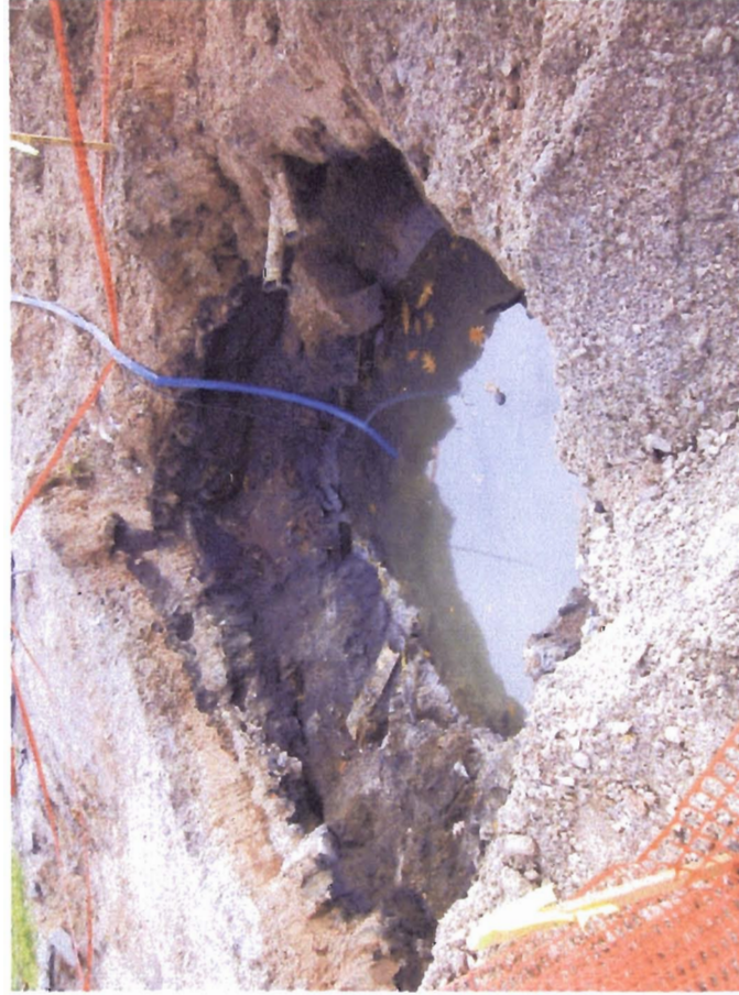
Photo 3: Photo of test pit TP-1 excavation where sample was collected along sidewalk.
