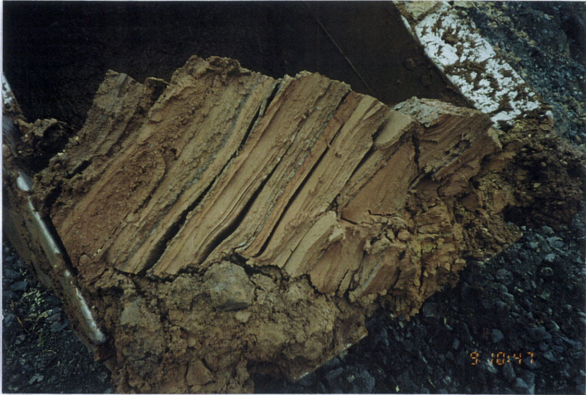
Photo 11: Horizontal layering of clay and silt soils on site.
