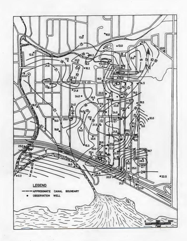
Figure 8. Contour diagram of thickness (ft) of clay.
