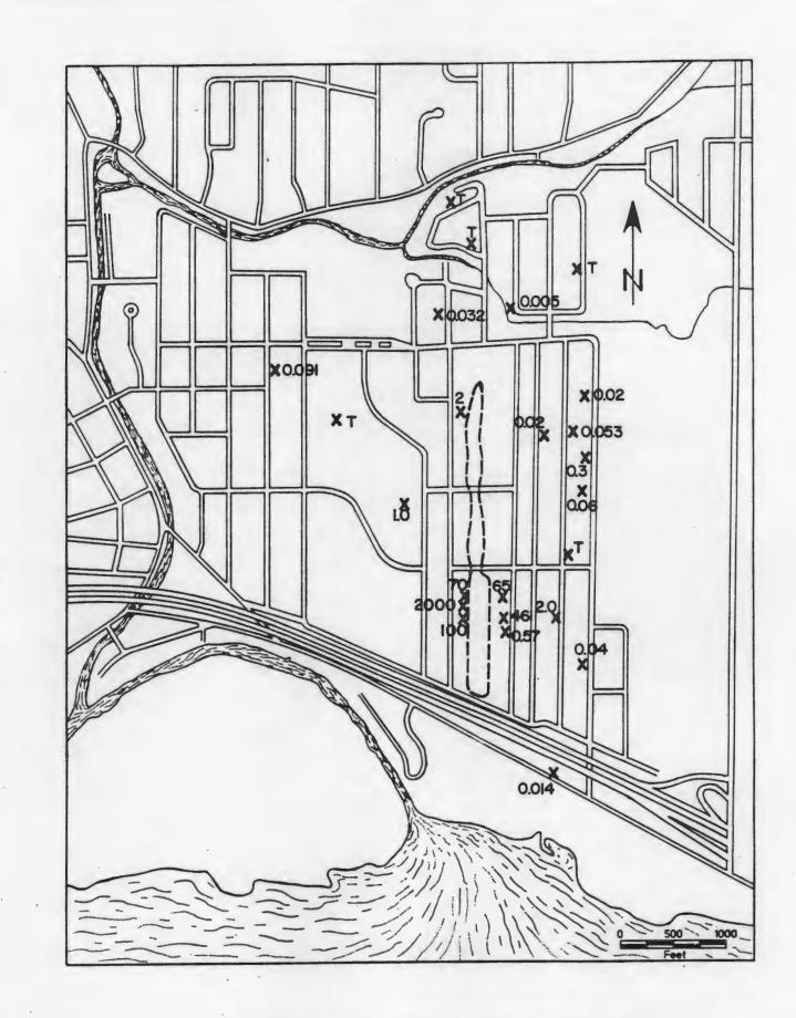
Figure 21. Concentrations (ppb) of  $\gamma$  BHC in sump samples.
