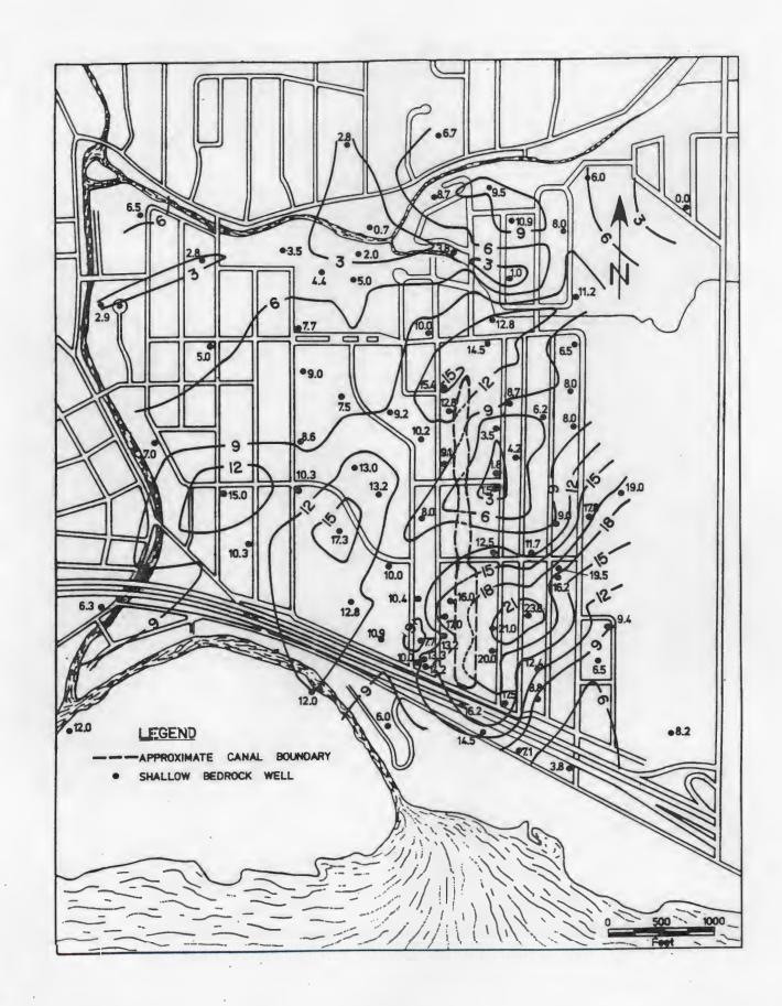
Figure 7. Contour diagram of thickness (ft) of till.
