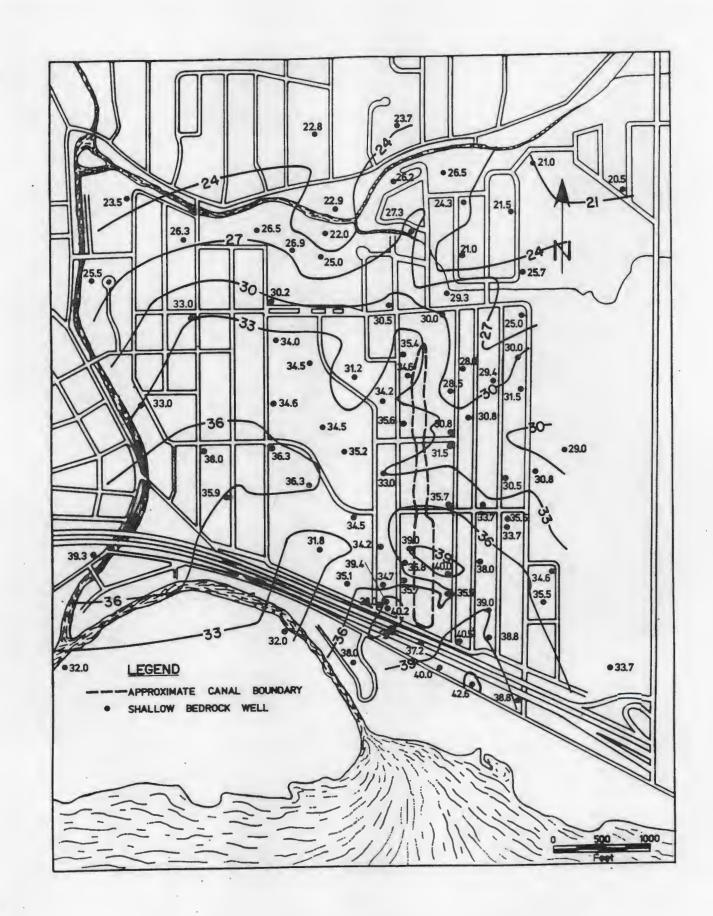
Figure 10. Contour diagram of total thickness (ft) of overburden.
