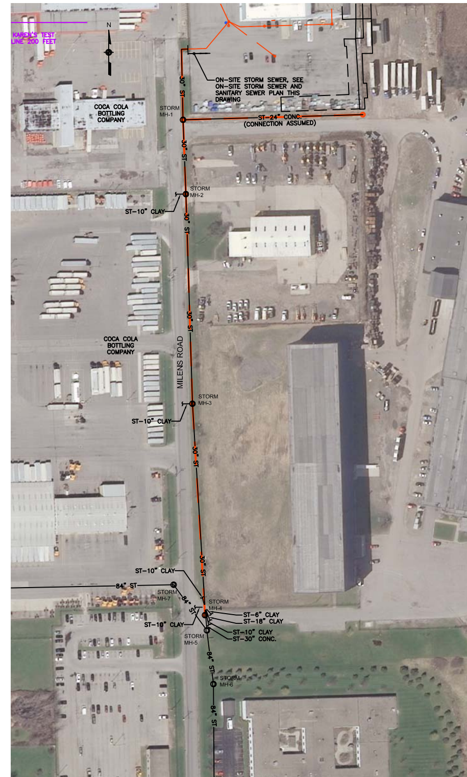
OFF-SITE STORM SEWER PLAN
