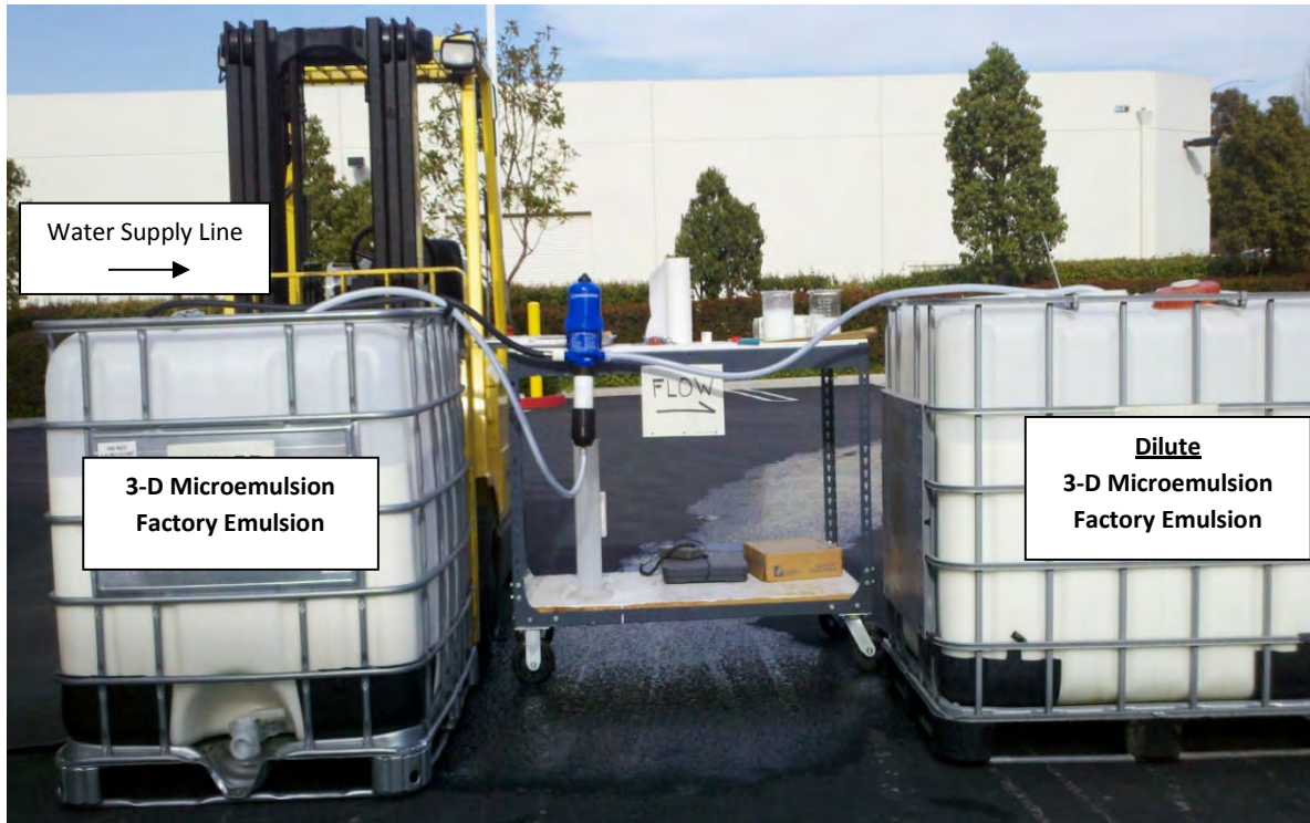
Dilution of the Factory Emulsified 3-D Microemulsion ® in a Batched Configuration
