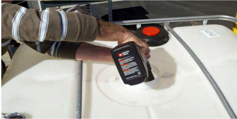
3-D Microemulsion ® Factory Emulsified Field Homogenization using a Cordless Drill Equipped with a Paint Mixing Attachment
