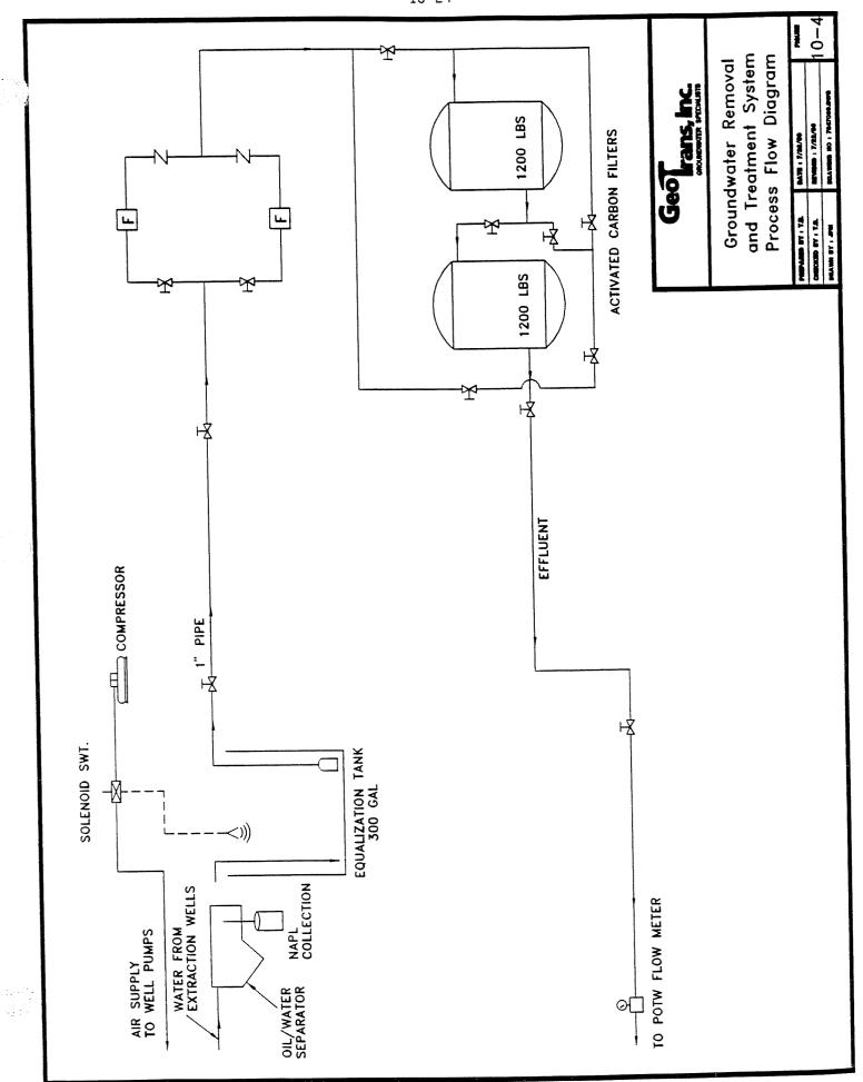
Extracting and treating the contaminated groundwater would reduce the toxicity and volume of the contaminated material and decrease the mobility of the plume. In addition, the extraction well system would ensure that the plume of contaminated groundwater was contained.
