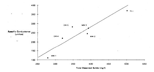
It should be noted that the instrument used to collect the specific conductivity measurements from the wells is the same one used for the temperature measurements. Since there is some suspicion as to the validity of the temperature results, the specific conductivity values must also be viewed with caution.
