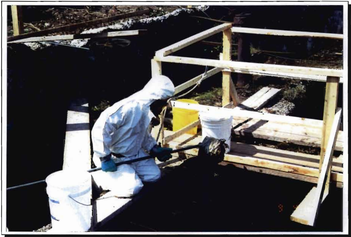
Photograph 2. Sampling contents of separator.
