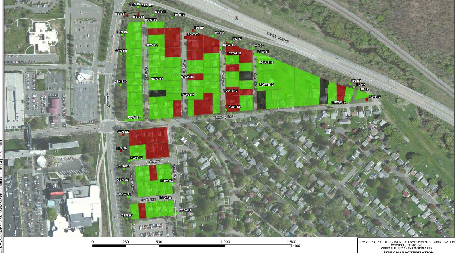
Exceedances of RSCOs in 4+ Feet Below Ground Surface (BGS) Soil Sample
