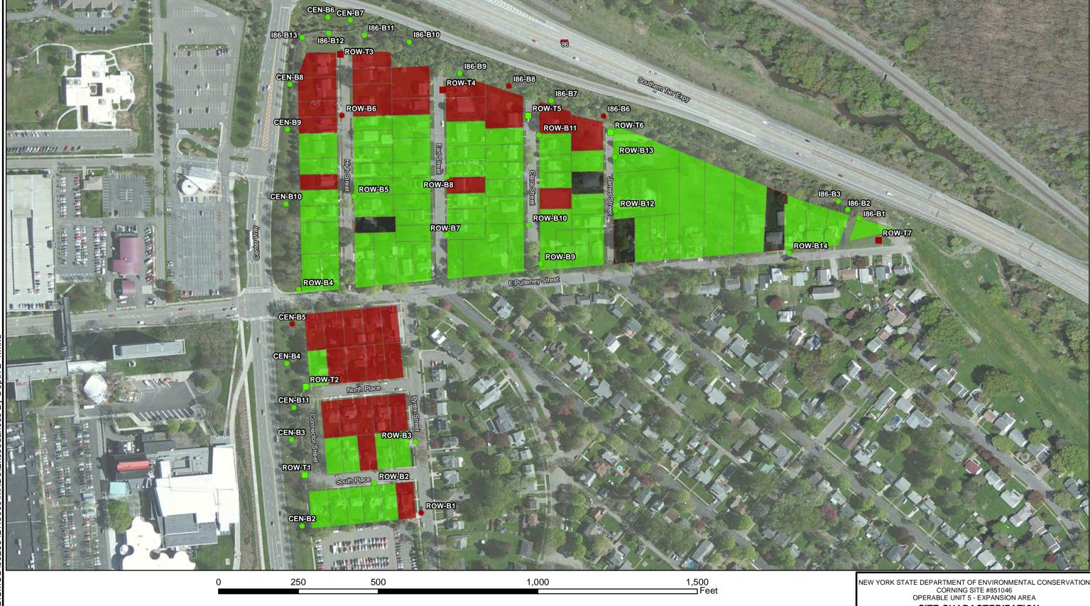
Exceedances of RSCOs in 2-4 Feet Below Ground Surface (BGS) Soil Sample
