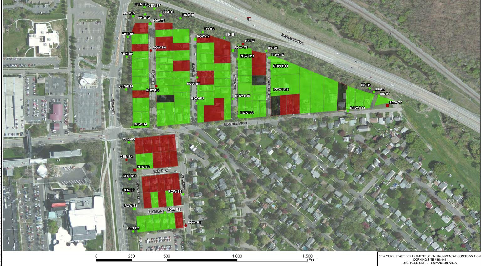
Exceedances of RSCOs in 0-2 Feet Interval Below Ground Surface (BGS) Soil Sample
