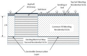
Diagram of the soil cover system installed in residential areas
