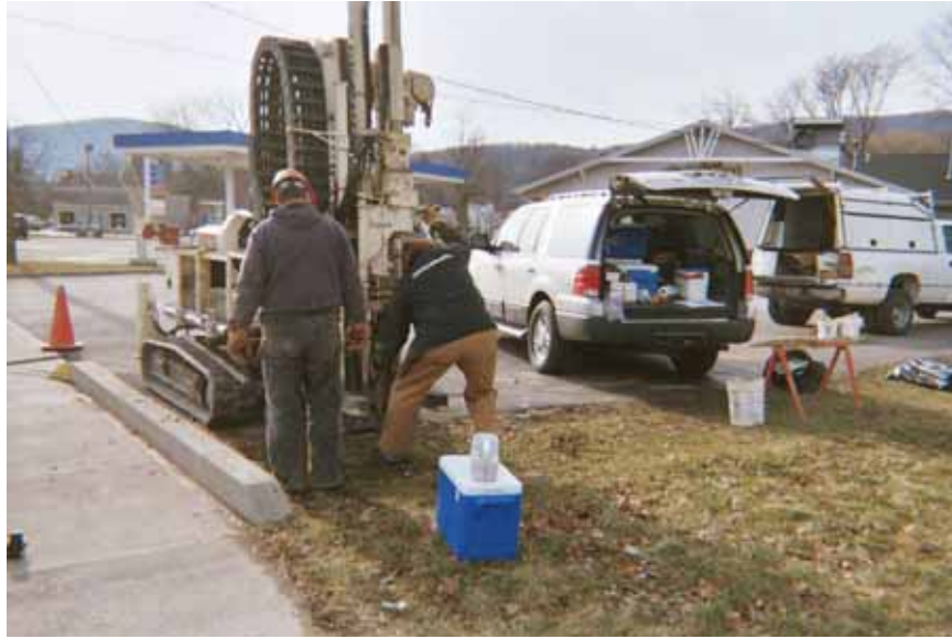
Date: 1/26/06 Subject: Direct-Push activities at the Former Depot Street Dry Cleaner Site boring DS-BH-02 Photographer: Stephanie Reynolds Smith
