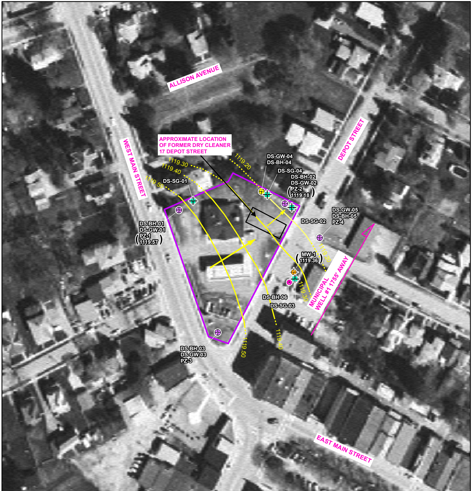
Figure 3-2 Former Depot St. Dry Cleaner Sample Locations and Groundwater Contours
