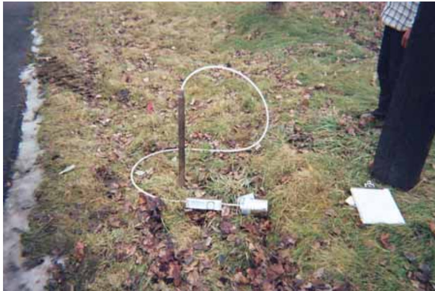
Date: 1/4/06 Subject: Typical soil gas sample collection set-up Photographer: Stephanie Reynolds Smith
