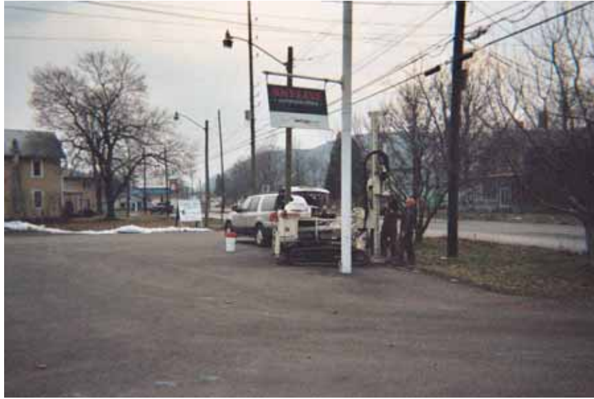
Date: 1/11/06 Subject: Direct-Push activities at the Former Loohns Cleaners Site boring FL-BH-03 Photographer: Jim Mays
