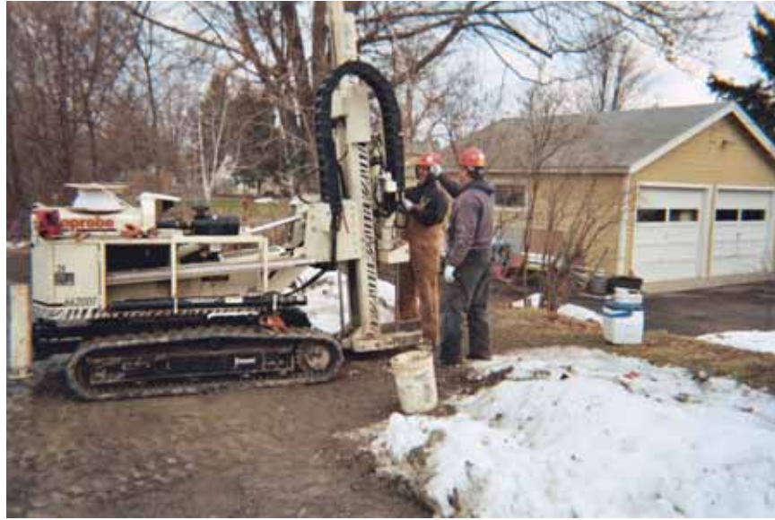
Date: 1/9/06 Subject: Direct-Push activities at the Former Loohns Cleaners Site boring FL-BH-01 Photographer: Jim Mays
