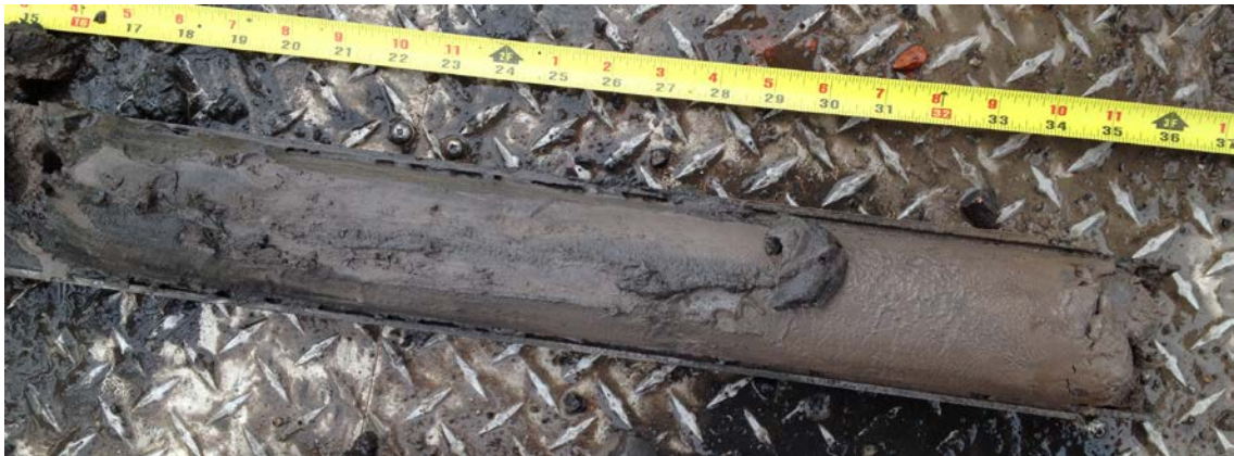
Undisturbed core sample from Gorham Street Finger area – GSD-2 DMU – Note Clast/gravel at bottom
