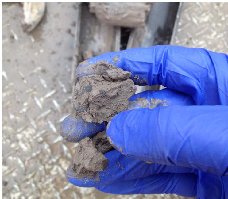
Typical Till material – with sub-angular clast ingrained throughout the interval
