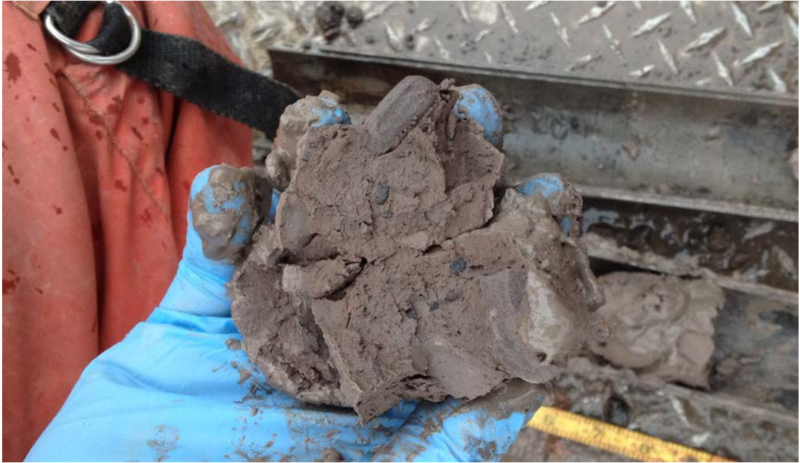
Typical Till material – with rounded and sub-angular clast ingrained throughout the interval
