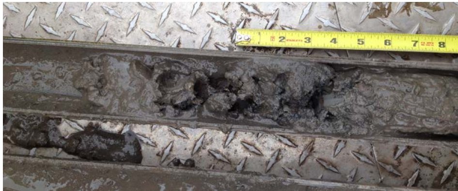
Brownish black Soft Sediment found in the Finger Area of Gorham Street Deposit (GSD-1)
