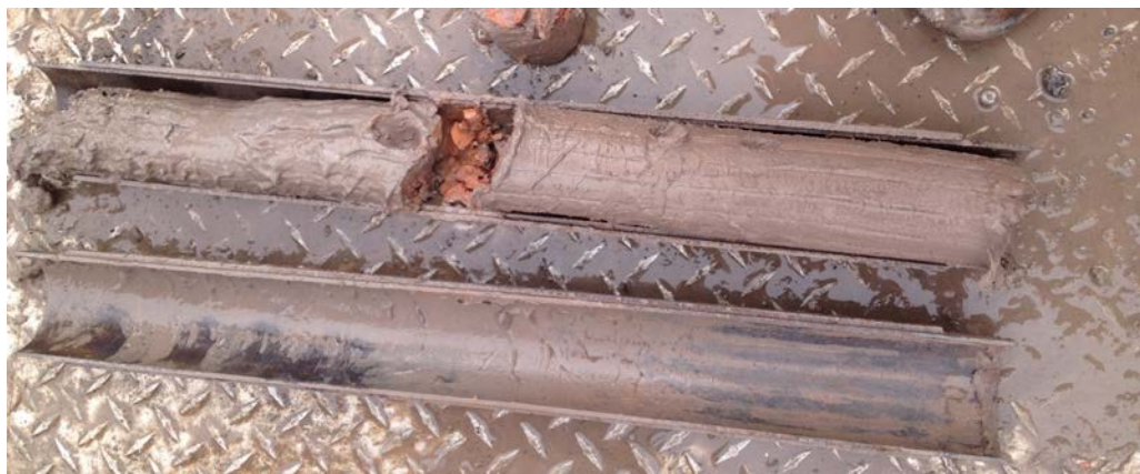
Fat Clay observed in Gorham Street Deposit (GSD-2) at CSC-03 with Red Brick in between
