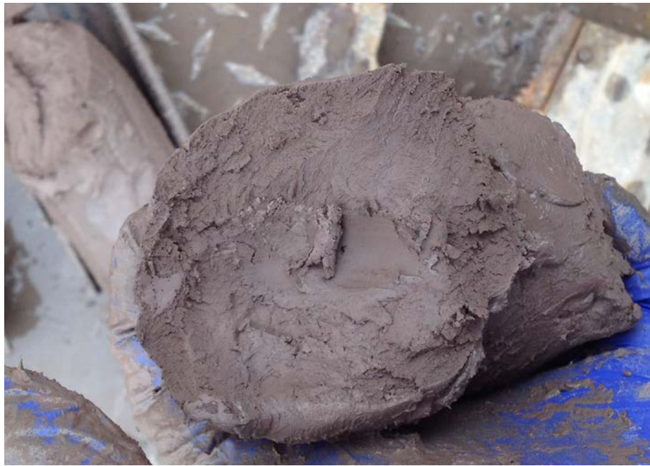
Dry – Typical Pale reddish brown Till material observed in Gorham Street and Downstream Deposit
