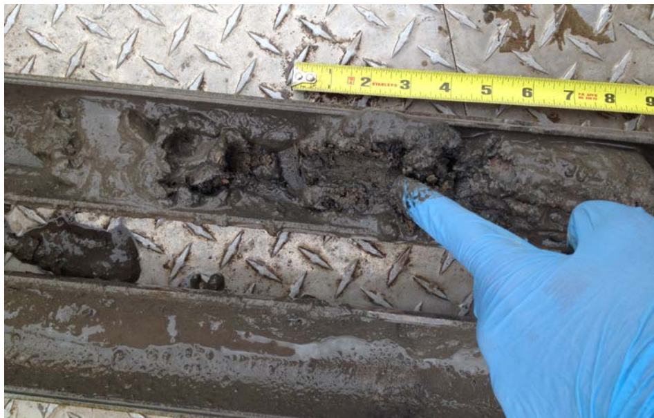
Typical Soft Sediment found in the Finger Area of Gorham Street Deposit (GSD-1)
