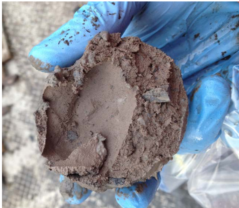
Typical Pale Reddish Brown Till material with Clast (Angular / Sub-angular) observed in the Gorham Street and Downstream Deposits
