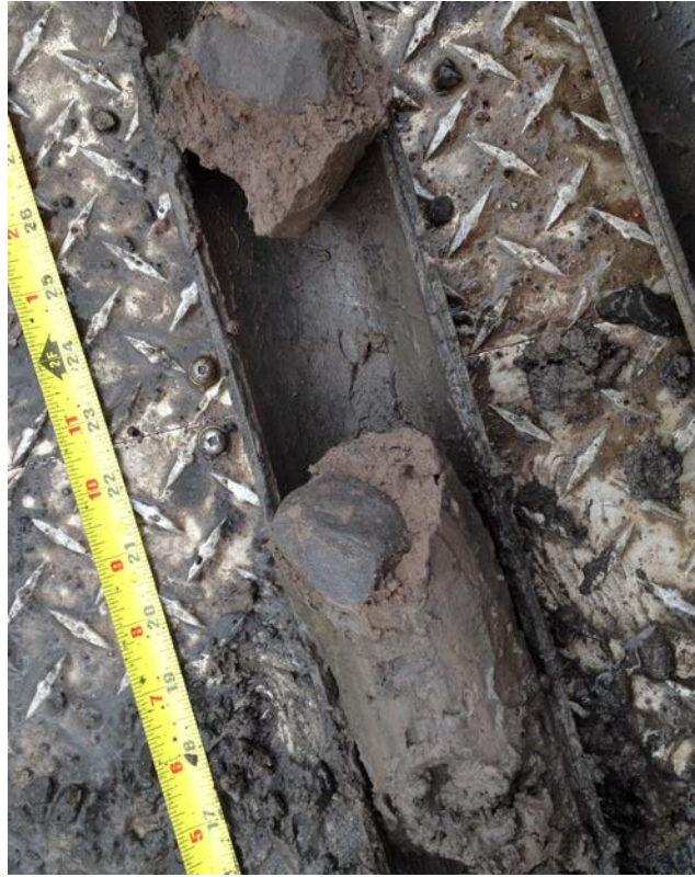
Typical Pale Reddish Brown Till material with large Clast / gravel (Rounded / Sub-angular) observed in the Gorham Street and Downstream Deposits.
