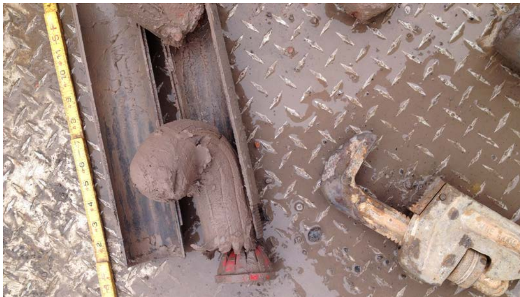
Highly Plastic / stiff fat clay at Gorham Street Deposit GSD-2
