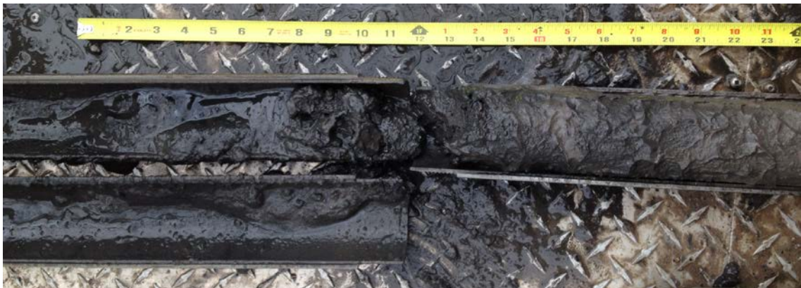
Typical Black, Very Soft Sediment observed in the Finger Area of the Gorham Street Deposit (GSD-1)
