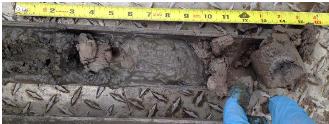
Soft Sediment / Compacted fine sand layer above the till material observed in Gorham Street Deposit (GSD-2)
