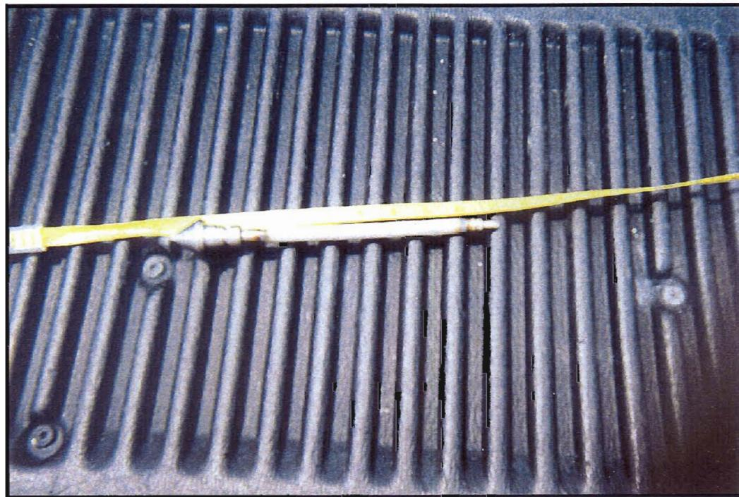
Photo 1: Photograph of a soil gas implant.
