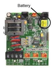
The battery cell is mounted in a socket on the right side of the main power board. Should the battery drop below 2.4 VDC in capacity, the display will illuminate a battery symbol on the left margin indicating a low condition. Additionally, the internal f rmware will set a f ag indicating the low
